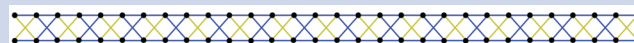
Figure 1. Graphical representation of a 60-qumode (vertices) quantum state, entangled as per the graph edges (blue and yellow). Each qumode act as a qubit and the quantum correlations from the preestablished entanglement can be used to implement universal quantum computing.
